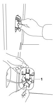
Reverse this procedure to insert the new LED light.
